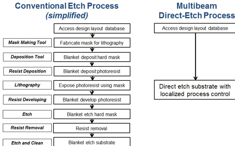
Fig.1: Comparison of (LEFT) the many steps needed to etch ICs using conventional wafer processing and (RIGHT) the two simple steps needed to do direct etching. (Source: Multibeam)
