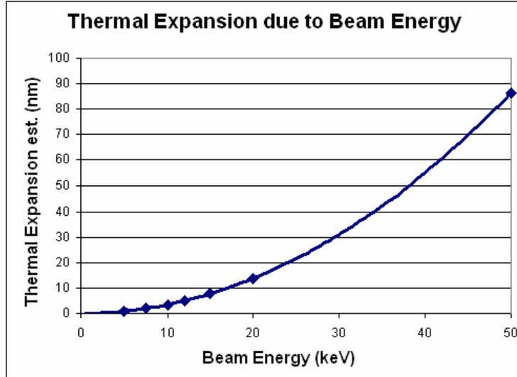
Figure 7. Thermal expansion of 300mm wafer due to e-beam energy.
