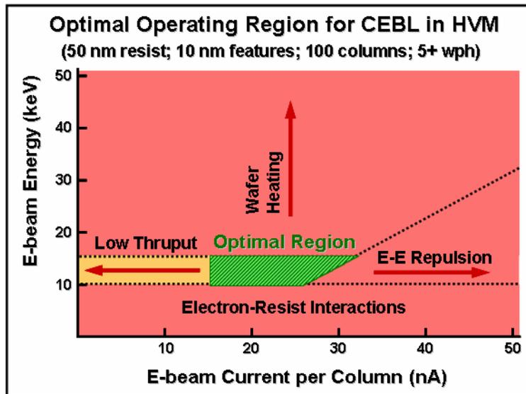
Figure 8. The optimal operating region for a typical column designed for CEBL ranges from 10 keV to 15 keV beam energy and 15 to 30 nA beam current per column.
