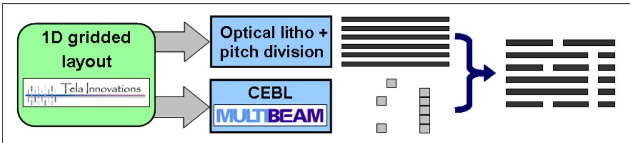
Figure 1: E-Beam and Optical lithography both have strengths and weaknesses. 1D layouts enable a complementary lithography approach that draws on the strengths of both Optical and E-beam lithography.
