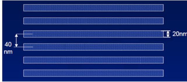
Figure 4: 20 nm line/space pattern with optical lithography and pitch doubling.<sup>7</sup>
