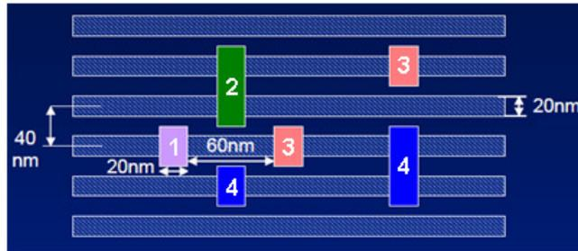
Figure 5: Intel approach for 20nm line/space. This can be accomplished with 4 optical cut masks, or 1 cut mask with EUV, or 0 masks with EBL.<sup>7</sup>
