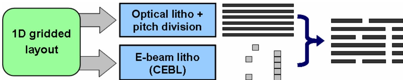
Figure 6: This shows Complementary E-Beam Lithography (CEBL) used hand-in-hand with Optical. A layout with 40nm pitch requires Optical litho with four “cut” masks, or E-Beam Lithography with zero “cut” masks.
