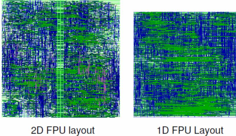
Figure 3: Comparison of chip size for 2D and 1D layouts of FPU (floating-point unit).
