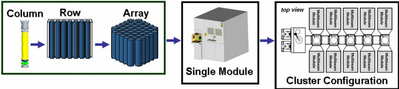
Figure 9. Multibeam scalable architecture. Multibeam optimizes a single column before building an Array of identical columns. A module with a single column array is capable of patterning 5 wafers per hour. A cluster tool is capable of patterning 50 wafers per hour.
