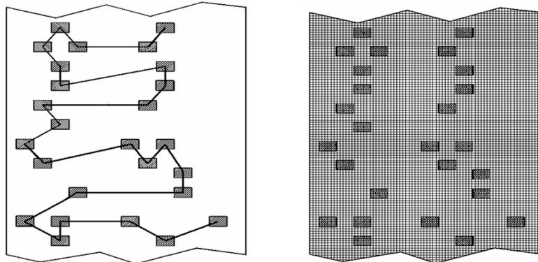
Figure 10: Comparison of Vector-scan and Raster-scan approaches. On left, the vector-scanned beam patterns an entire field with 45 high-speed flashes as it jumps over empty areas between flashes. On right, > 90% of beamlets are “off” while > 900 pixels are flashed for the same pattern.
