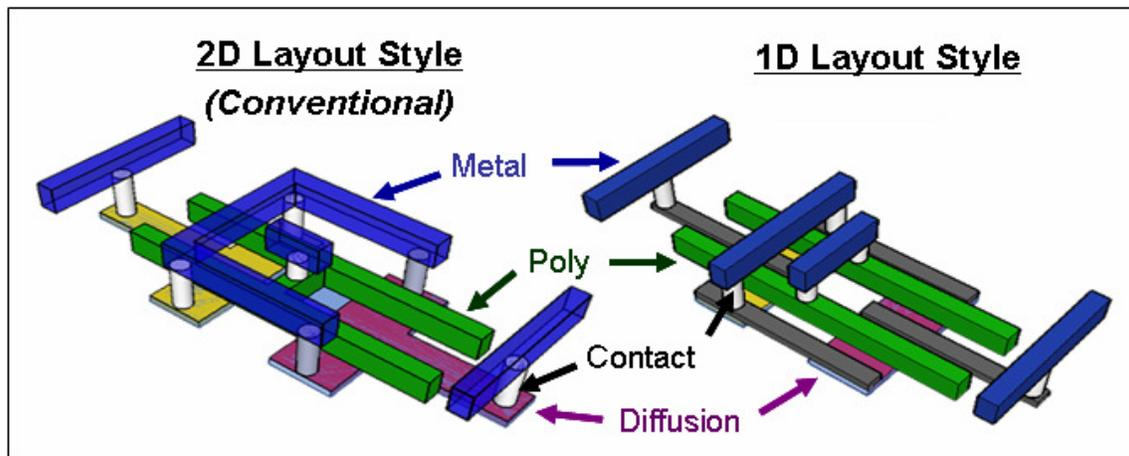
Figure 2: Conversion of CMOS layout from traditional 2D design to 1D layout.
